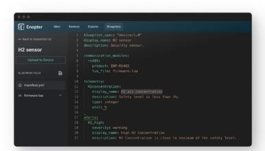
YAML-based Enapter Blueprints let you easily create integrated templates for UCMs, Intelligent Gateway, Enapter Cloud and user apps.
