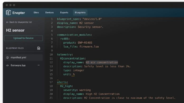
YAML-based Enapter Blueprints let you easily create integrated templates for UCMs, Intelligent Gateway, Enapter Cloud and user apps.
