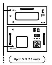
In order to manage the hydrogen purge in a simple way, simply connect as many devices together as needed.
