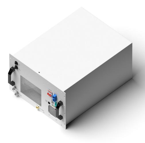
This is the DC version of Enapter's patented anion exchange membrane (AEM) electrolyser- a standardized, stackable and flexible system to produce on-site hydrogen. The modular design – paired with advanced software integration – allows set up in minutes and remote control and management. Stack this electrolyser to achieve the required hydrogen flowrate.
