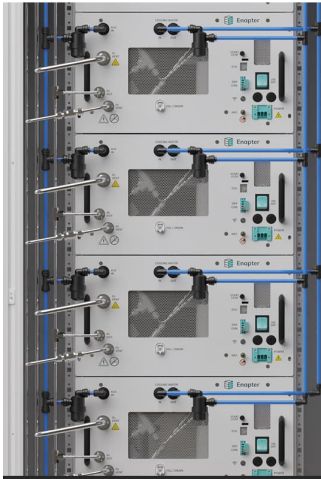
Dry Con daisy chain with two electrolyzers and Emergency Switch
