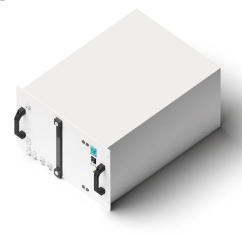
Enapter's Water Tank provides storage for 38 litres of clean water for the AEM electrolyser. The water tank is rack mountable into a standard 19" cabinet. The tank contains a conductivity sensor and a pump system to supply up to 11 AEM electrolysers with clean water.
