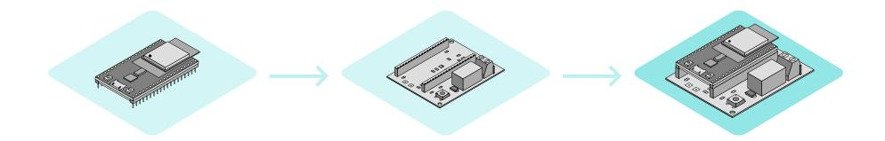
Purchase a common Espressif ESP32-DevKitC board <u>More info</u> Order and assemble an ENP-KIT shield board from a variety of available opensource documentation from GitHub More info Assemble boards together and power them using your computer USB port
